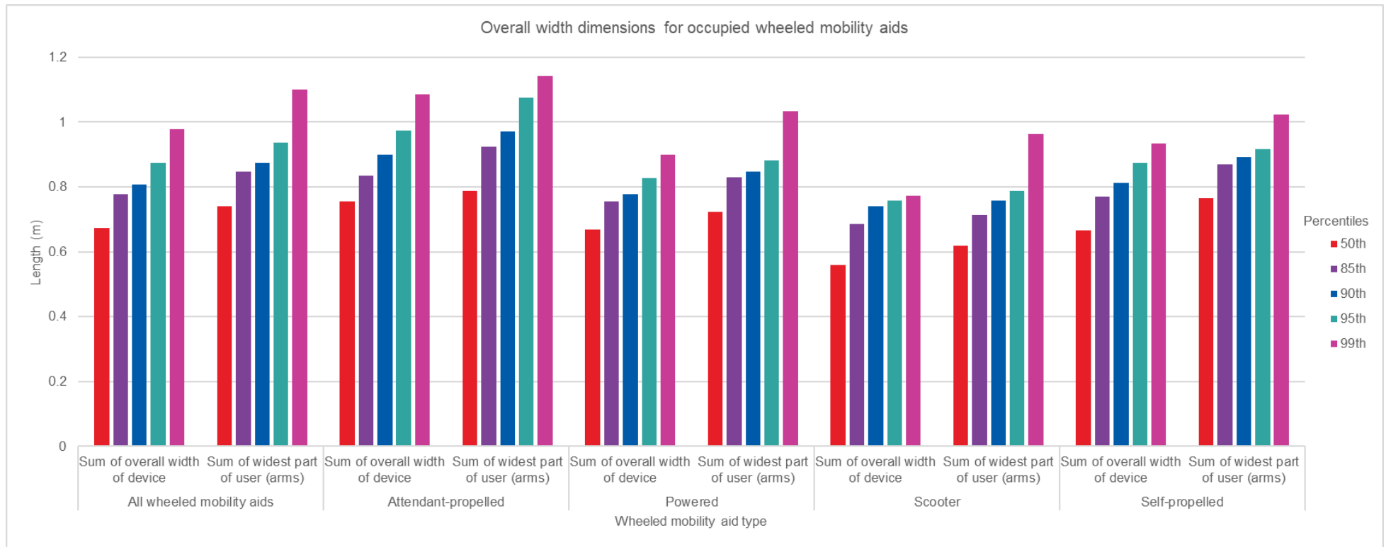
Figure 8. Key dimensions for occupied wheeled mobility aids – by type of wheeled mobility aid.
